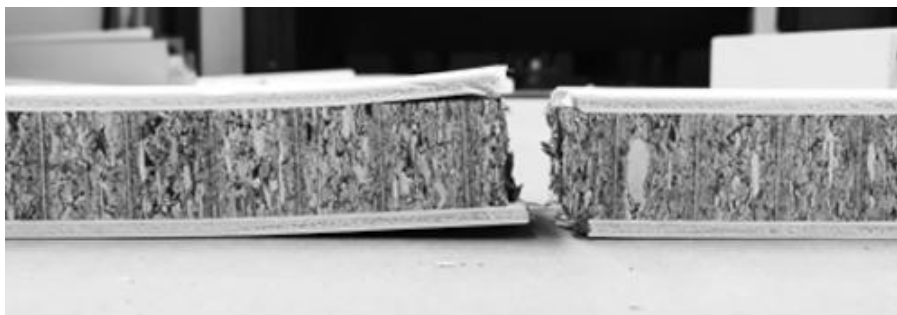
Fig. 7. Residual deformation in the failure zone of a PL 4 series element
