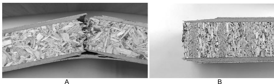
Fig. 5. Damaging of \text{MDF}_v specimens under bending stress: A - Elements from Series AA; B - Elements from Series PP
