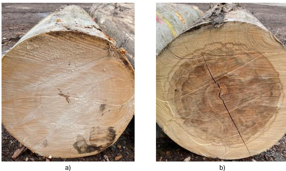
Fig. 1. Beech log sections: a) without red false heartwood, b) containing red false heartwood
