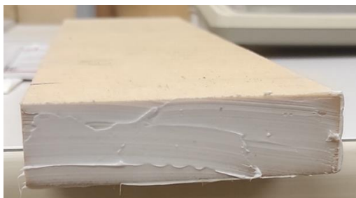
Fig. 3. Drying sample with silicone layer
